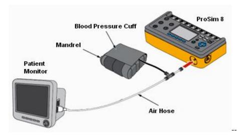
Fig. 8 Non-Invasive Blood Pressure Test Connections
