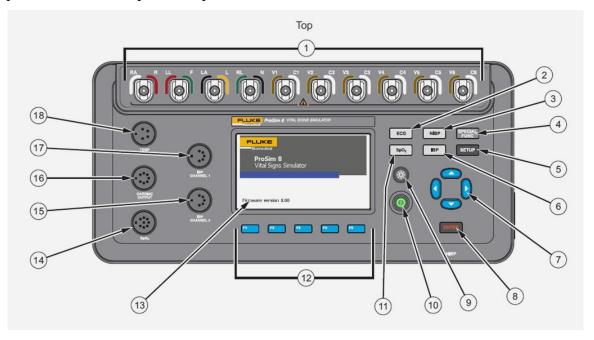
Fig. 5 <u>Vital signs simulator ProSim 8</u> (Top-Panel Controls and Connections)
