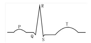
Fig. 2 Standard ECG waveform
