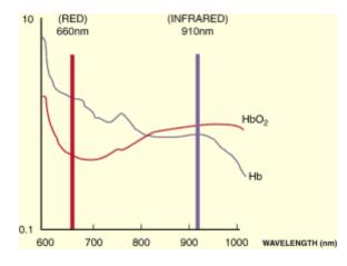
Figure Absorption spectra of Hb and HbO<sub>2</sub>.
