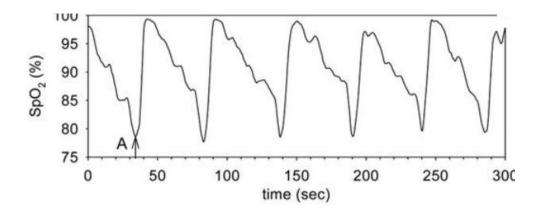
Figure Typical pulsatile signal detected when light is shone through a finger.
