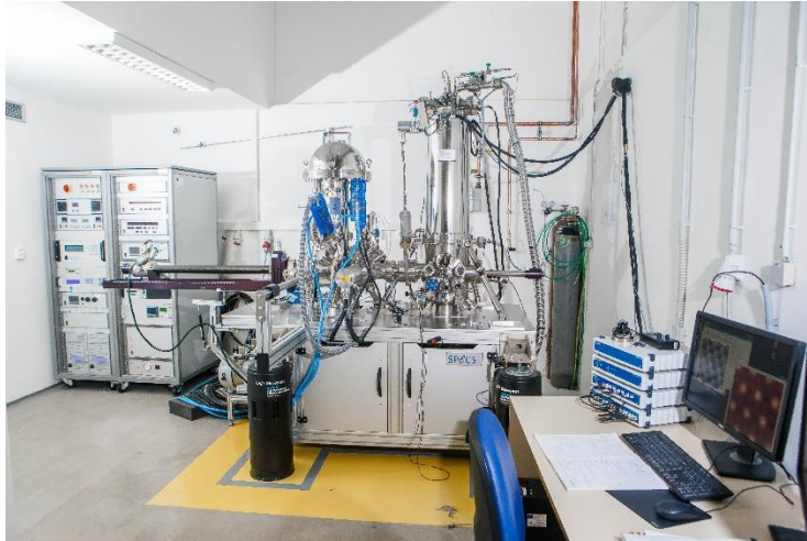
Obr. 3: Our cryogenic scanning tunneling microscope in ultra-high vacuum.
