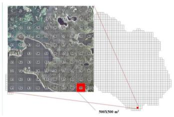
Fig. 3 Principles of selection of sub-quadrates in 5 x 5 km quadrates. In this case, the  $99^{th}$  500 x 500 m monitoring sub-quadrate is marked in the  $99^{th}$  quadrate.
