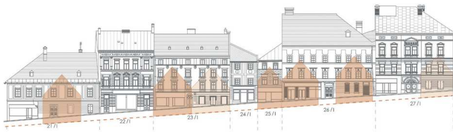
Schematic silhouette of the building structure from the 13th century, inserted into the current facades (A. Kmeťa Street)
