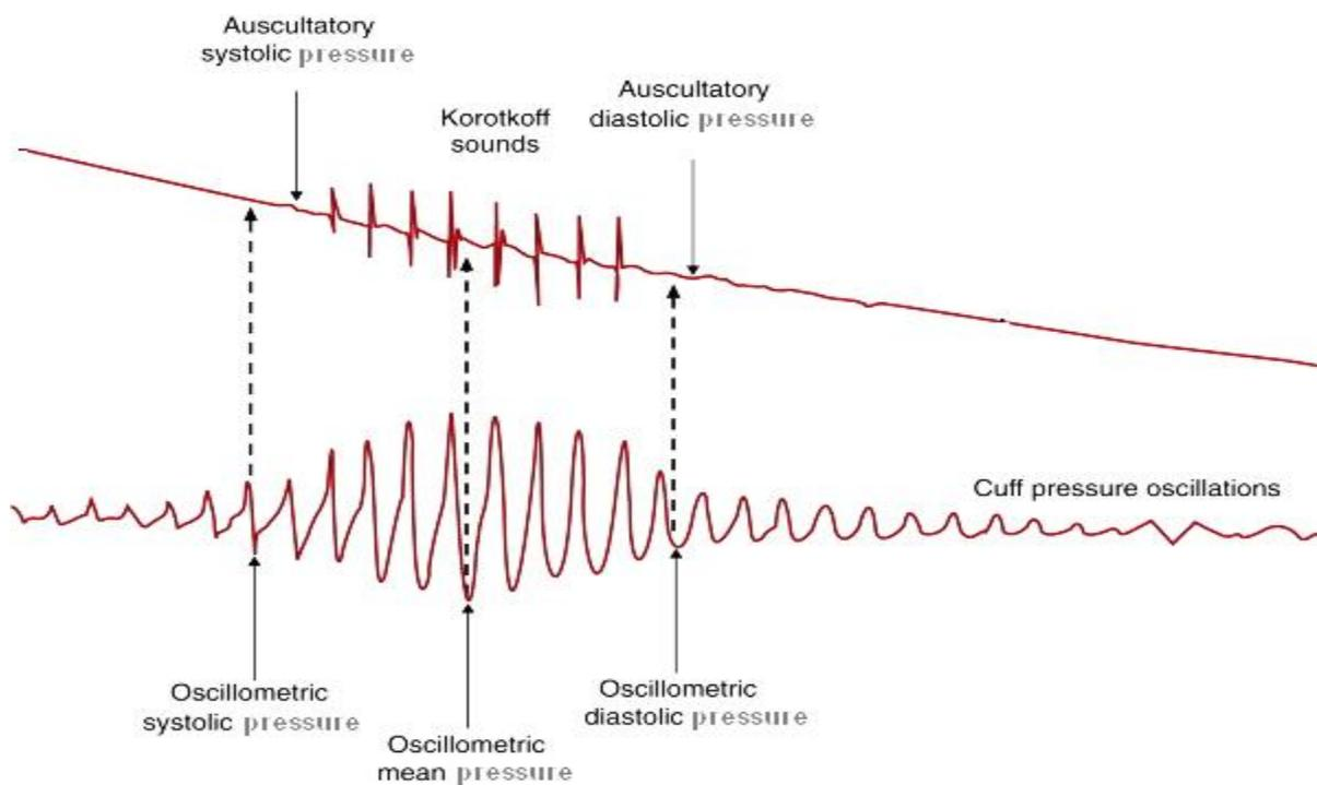
**Fig. 3** Measurement of systemic arterial pressure according to oscillometric method
