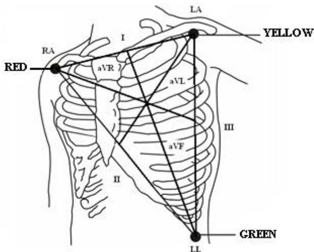
**Fig. 1** Einthoven's triangle and standard bipolar leads
