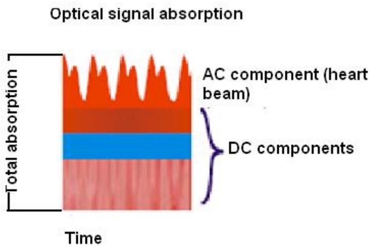
Figure The AC and DC pulsatile signals.
