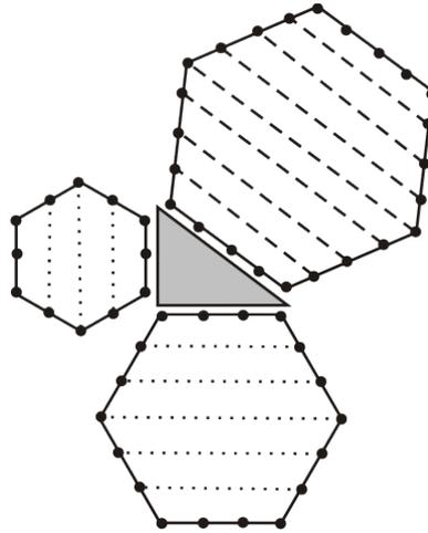
Figure 10: The longitudinal hatching length in the case  $a = 3, b = 4, c = 5, (r = 1)$  and  $m = 6$
